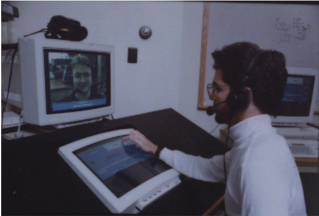
FIGURE 4. JANUS-II Speech Translator in a Video Conferencing Environment. Translation appears visually as subtitles as well as by synthetic output. The system is controlled by buttons on a touch sensitive display. Vocabulary size is between 1000 and 3000 words per language. Translations are obtained in 2-3 times real-time
