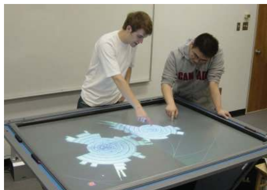
Fig. 1. The hardware setup for our collaborative information visualization application. Two simultaneous pen or finger inputs are possible.
