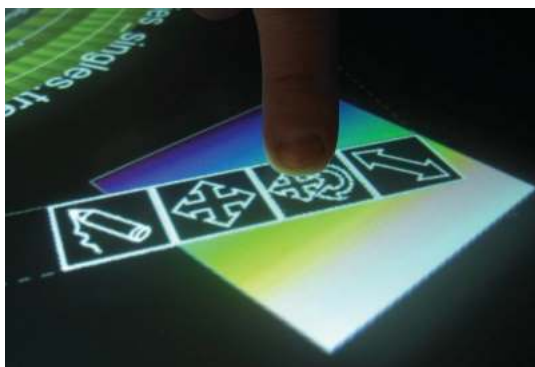
Fig. 8. A visualization plane is dropped on a ColourChanger widget that changes the colour scale with which the tree is displayed.
