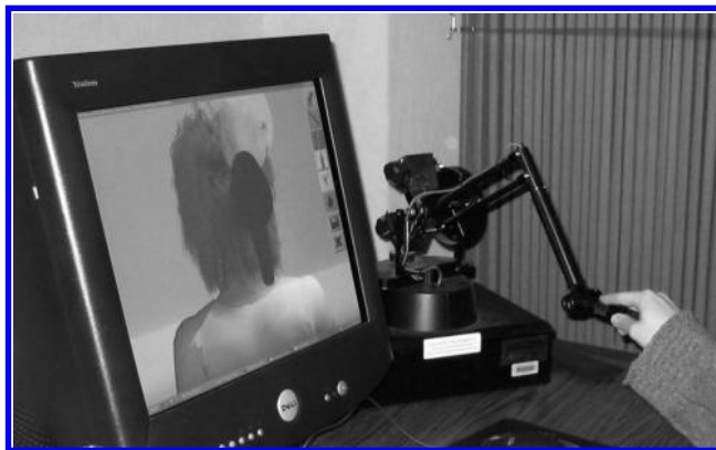
Figure 2. User interface: PHANToM provides 3D user input and 2D menu buttons are labeled with icons to show applications.
