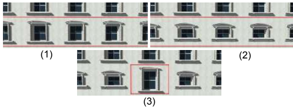
Figure 13: Sequence showing hierarchical modifications. (1) A shape representing a floor is selected. (2) The parameter windowHeight is modified - all shapes on lower levels are automatically modified (3) Selecting a specific shape allows overriding the parameter on a lower level.
