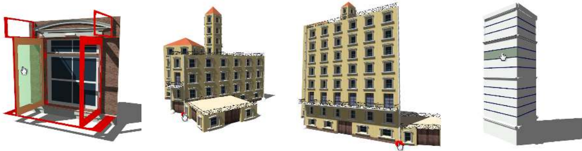
Figure 1: Screenshots from our real-time editor for grammar-based procedural architecture. Left: Visual editing of grammar rules. Middle left: Direct dragging of the red ground-plan vertex and modifying the height with a slider creates the building on the middle right. While dragging, the building is updated instantly. Right: Editing is possible at multiple levels, here the high-level shell of a building is modified.
