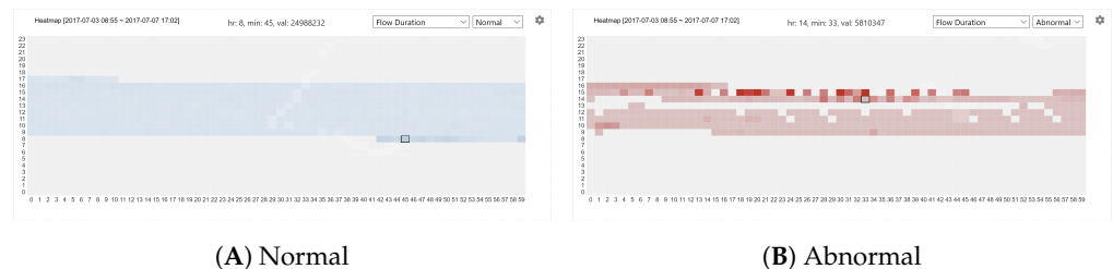
Figure 5. Heatmap visualizations of the attribute (i.e., Flow Duration). The vertical and horizontal axes in the heatmap view indicate hour (0~23) and time (0~59) information, respectively. Each heatmap cell holds an average value of the selected attribute within a specified time. In the view, blue and red colors are used to indicate normal and abnormal activities. Gray color represents no activities.
