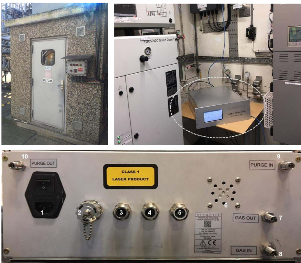
Figure 5. The sensor system in the analyzer house at Preem refinery (top images). The overview of connection ports on the rear panel (bottom image). The corresponding numbers refer to: (1) power inlet 230VAC 50Hz, (2) service ethernet port RJ-45, (3),(4),(5) I/O cable glands, (6) ventilation outlet, (7),(8) sample gas inlet/outlet, (9),(10) purge inlet/outlet.
