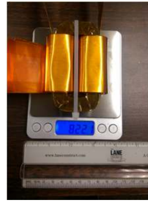
FIGURE 10. The photo of an ICT hardware for the 100-kW PV inverter application.
