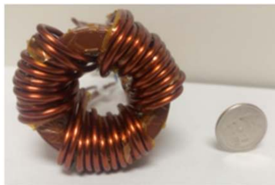
FIGURE 19. CM choke for ground leakage current suppression. 240 \mu H @100 kHz, 229 g.
