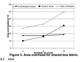
The area consumed by the shared bus fabric comes from wiring and interconnection-related logic, as described in Section 4. Wiring overhead depends on the architected buses and the control wires that are required for flow control and arbitration. Control wires are needed for each multiplexor connected to the buses and signals to and from every arbiter. Flow control wires are needed from each queue to the units that control traffic to the queue.
