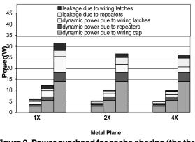
Figure 9. Power overhead for cache sharing (the three bars, left to right, correspond to 2-way, 4-way and full sharing).
