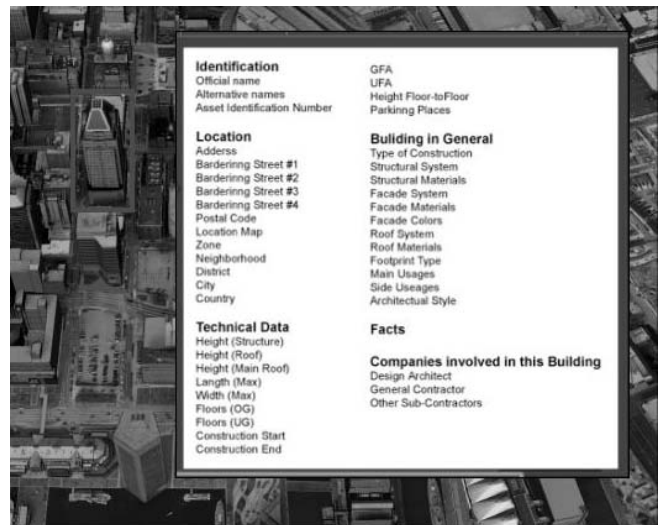
Figure 3. CIMS ® possess the ability to select simulation entities and attach key information.
