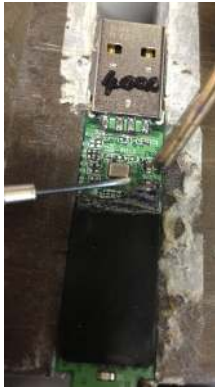
Fig. 4: Epoxy removal of Kingston DT 5000 with screwdriver
