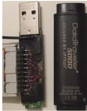
Fig. 5: Eavesdropping the bitstream of Kingston DT 5000 with opened case
