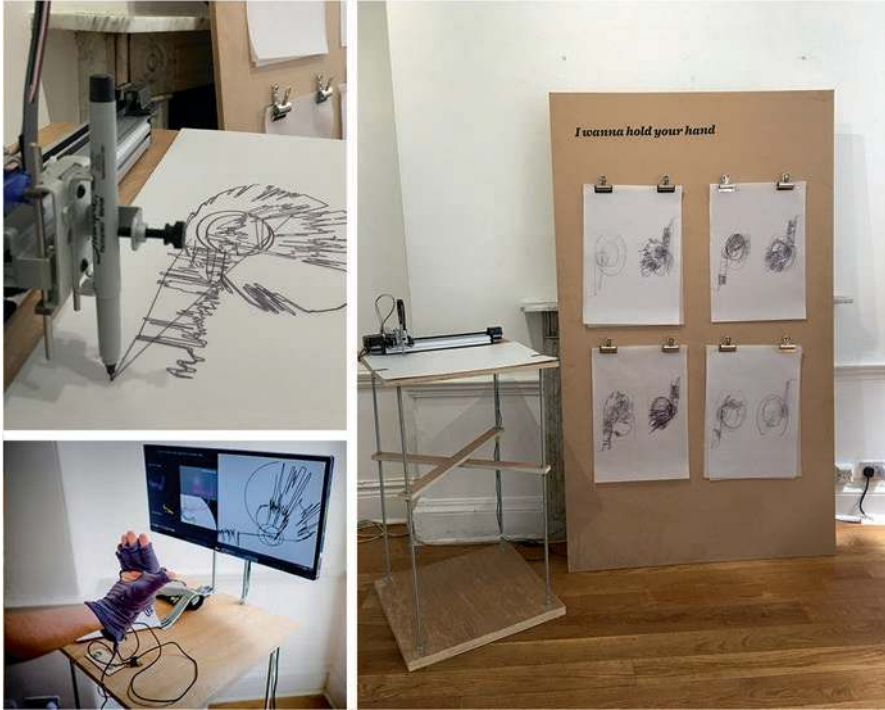
Fig. 4.2 The Remote Contact exhibition ‘I wanna hold your hand’ artefact, traced the experience of a joint walk, holding hands, via a pair of digitally-enabled gloves. Embedded galvanic skin and pressure sensors and GPS linked to an Arduino plotter that mapped the data collected. (Photo Credit Ed Waring)
