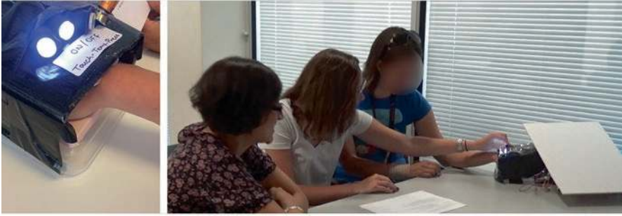
Fig. 4.4 The participants use the ‘heat dial’ of an early prototype Tactile Emoticon device to regulate the temperature of the tactile message
