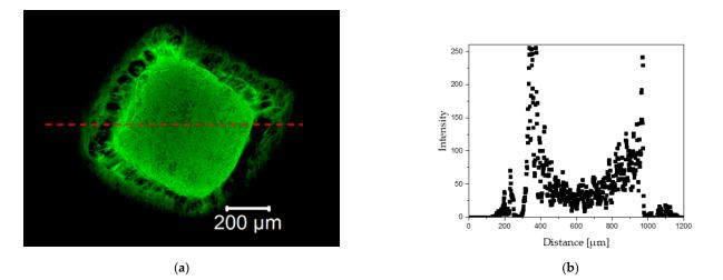
**Figure 9.** One-hundred-and-eighty second influence of the proton beam on tissue autofluorescence: (a) autofluorescence and line scan on fluorescence images; (b) intensity of light excited in autofluorescence—increase/decrease of autofluorescence at the proton over burning site.
