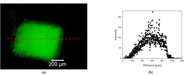
**Figure 8.** Two second influence of the proton beam on tissue autofluorescence: (**a**) autofluorescence and line scan on fluorescence images; (**b**) intensity of light excited in autofluorescence—increase of autofluorescence at the proton burning site.
