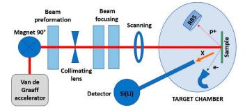
**Figure 3.** Experimental setup of the Cracow's scanning nuclear microprobe providing source for proton beam for sample irradiation.
