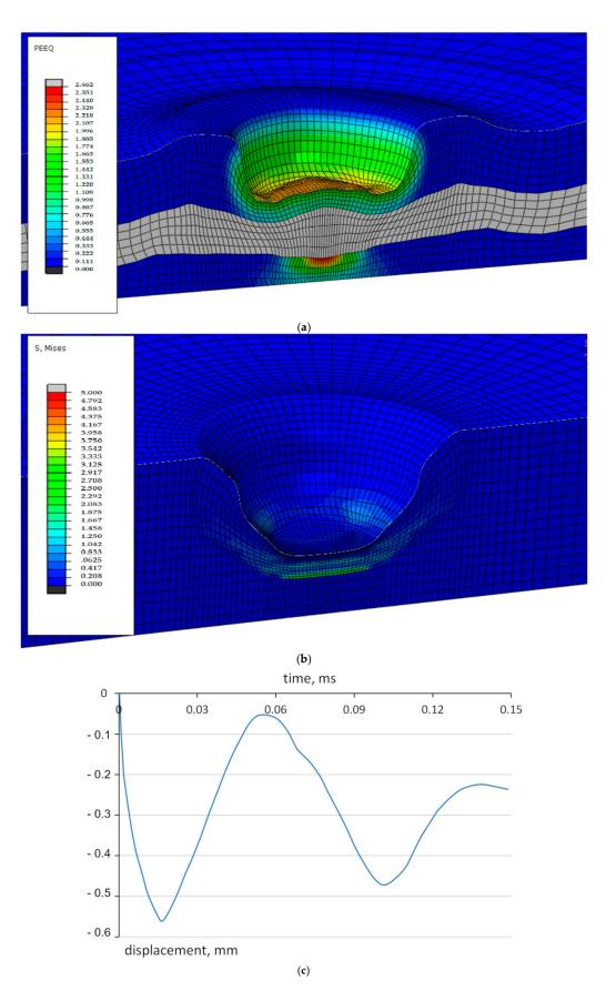
**Figure 4.** Results of 3D finite element three-layer tissue of animal origin model: (**a**) effective strain distribution—side view in a selected cross-section; (**b**) effective stress distribution—side view in a selected cross-section; (**c**) graph of displacement of central node versus time.
