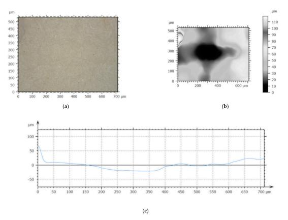
**Figure 5.** Tissue topography: Z—displacement, mm for animal-origin sample models; (**a**) the surface; (**b**) height map; (**c**) profile [53].
