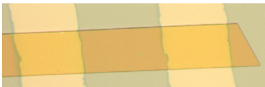
Figure 2.5 Electrostatic bonding of a rubrene single-crystal to a pre-fabricated transistor template with an \text{Al}_2\text{O}_3 dielectric layer and Au source and drain electrodes. Figure with permission from [68].
