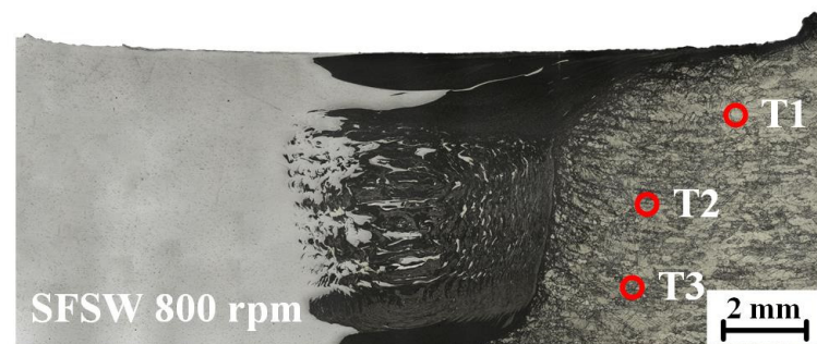
Figure 8. Diagram of the thermocouple position.
