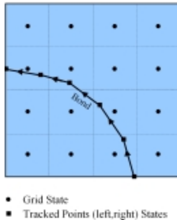
FIG. 2.1. A representation of the grid for a front tracking computation. The solution is represented on the union of a spatial finite difference grid and a dynamic grid that follows the fronts.
