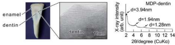
Fig. 16 Direct evidence of the formation of nano-layered structure on dentin (left) was provided by TEM (middle), and also by thin film X-ray diffraction of 10-MDP-dentin samples (right) 10 .
