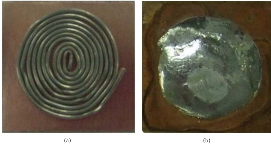
FIGURE 1: Appearance change of (a) a coiled SAC305 solder wire into (b) a solid SAC305 solder on the Cu substrate during solder reflowing.
