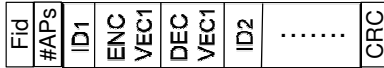
Figure 10: The metadata in a DATA+Poll frame. This metadata is broadcast by the leader AP alone to inform the clients in a downlink transmission group of their decoding vectors and the other APs of their encoding vectors.
