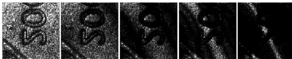
Figure 8. Build-up of axial resolution by superposition of holographic images of a penny using a range of wavelengths with N = 1, 2, 4, 8, and 20.
