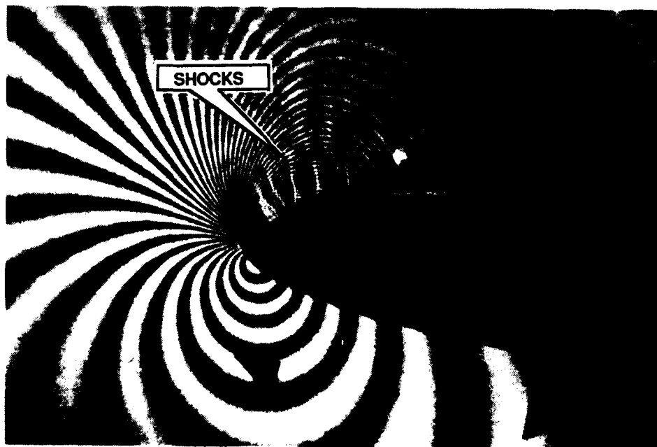
Fig. 4. Multiple Shocks over a Rapidly Pitching Airfoil, M = 0.45 , \alpha = 12.6^\circ , \alpha^+ = 0.0313 .
