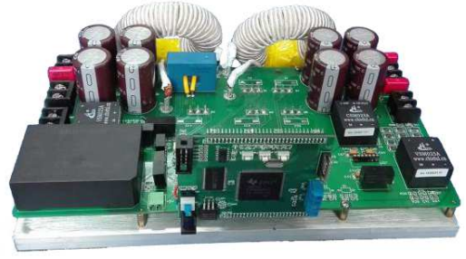
Fig. 9 The experimental prototype of the interleaved switched-capacitor bidirectional DC-DC converter.
