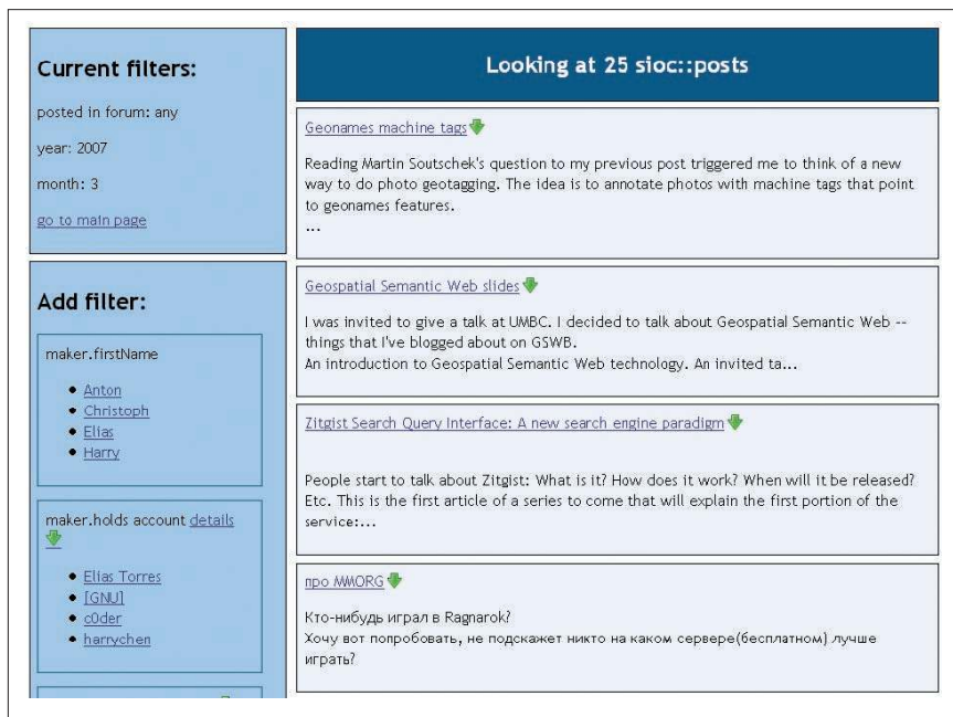
Figure 5. Faceted exploration of SIOC RDF data. The SIOC explorer lets users browse a broad view of disparate information in an integrated way.
