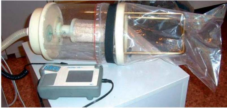
Figure 5 A laboratory image representing the Rebreather Hypoxytron® (Ukraine) device, which is capable of buffer reservoir volume regulation for individual hypoxia dosage (Photo taken by T.V. Serebrovskaya). (A color version of this figure is available in the online journal.)
