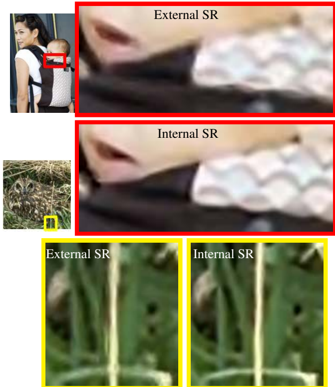
Figure 8. Super Resolution using External vs. Internal examples. External super-resolution exhibits more hallucinations and blur artifacts. More results can be found in www.wisdom.weizmann.ac.il/~vision/SingleImageStatistics.html
