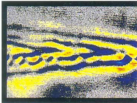
FIGURE 3. Vertical displacement \xi of the lee wave in a horizontal plane at |z|=3R below the centre of the sphere, for F=10/\pi and Re(1)=253 ( R=1.12 cm, N=1.17 rad/s.) (a, b) Experimental visualization at Nt=0 and 11.7; (c, d) calculated from linear theory at Nt=0 and 11.7. The scale is 46.5R \times 32R . Increasing downward motions (resp. upward motions) are colour coded from yellow to red (resp. dark blue to light blue). The sphere or source is moving from left to right in the x -direction.
