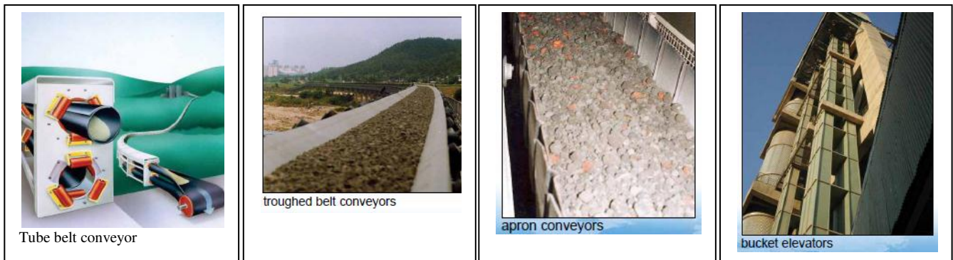
Figure 29. Mechanical transport systems (Hock 2008)
