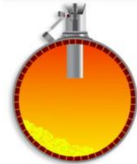
Figure 33. Cadence's mid-kiln fuel injector technology (Cadence 2012a).
