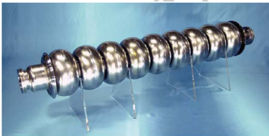
FIGURE 3.6-3. A low loss nine cell prototype RF structure under development.
