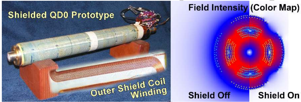
FIGURE 2.7-6. Prototype of QD0 quadrupole and its active shield (left); calculated field pattern with and without activation of the shielding coils (right).
