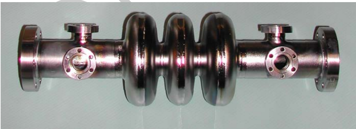
FIGURE 2.7-9. Photo of a 3.9GHz 3 cells deflecting cavity built at Fermilab, which achieved 7.5MV/m.
