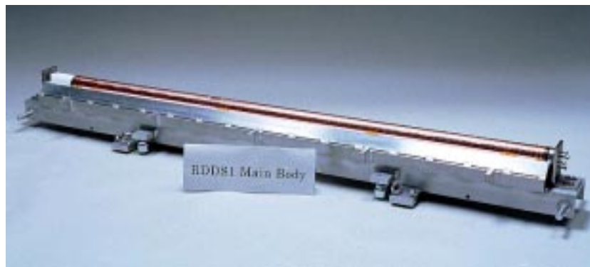
Figure 7.29: Completed RDDS1 disk stack after diffusion bonding.
