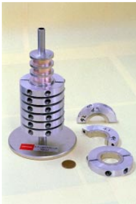
Figure 5.8: Prototype of Toshiba PPM magnetic circuit.
