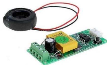
Figure 14. AC Power Sensing Device.
