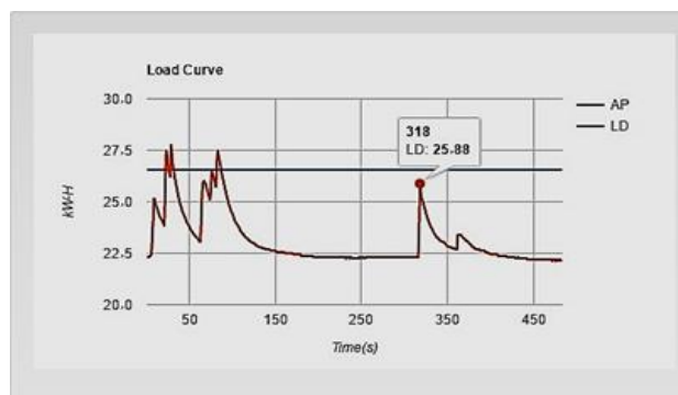
Figure 10. Monitoring of the Available Power and Load Demand.
