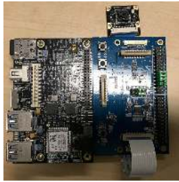
Figure 5: Smart camera setup. The ultra96 MPSoC with the camera connected to the extension board.
