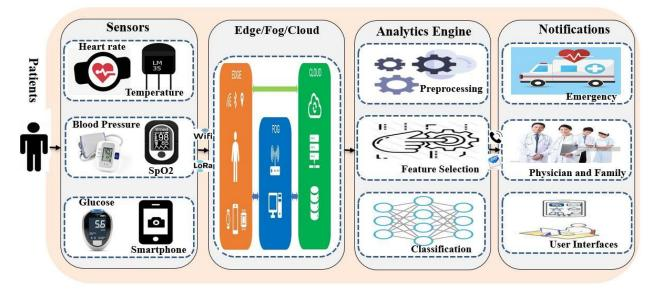
Fig. 5. A general pipeline of IoT-based smart healthcare systems. The sensors (heart rate, temperature, blood pressure, SpO2, glucose, and smartphone) collect the data from the real-time healthcare environment. Some of the data are processed in edge/fog server and the major data analysis occurs in cloud server where the data analytics engines predict the patient status. The emergencies, families, and physicians receive the patient's condition and take further required actions.
