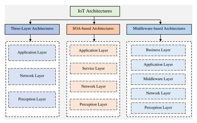
Fig. 3. Most common and frequently used IoT architectures that incorporate the three-layer architecture, SOA-based architecture, and middleware-based architecture.
