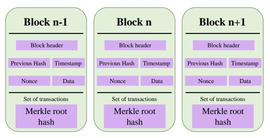
Figure 12. Basic structure of blockchain block.
