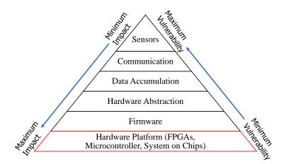
Figure 9. IoT devices attack pyramid based on effects and vulnerabilities.
