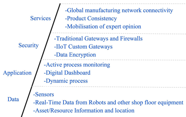
Figure 5. a proposed Industrial IoT architecture by [75].
