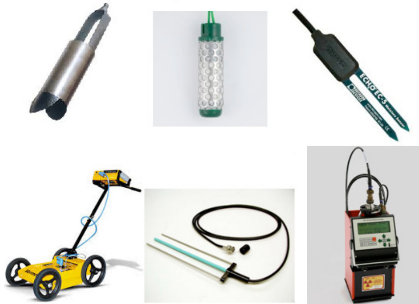
Figure 3: Soil moisture sensors: Top row: Gravimetric <90>, resistive (Watermark) <50>, capacitance <17>, Bottom Row: GPR <97>, TDR <128>, neutron probe <91>.
