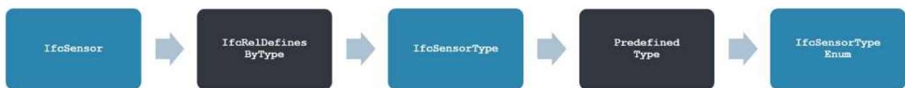
Fig. 2 Associating sensor types to IfcSensor instances using IFC4
