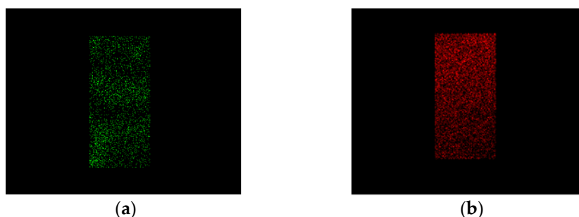
Figure 5. 50/50% v/v A/G aerogel maps: (a) Nitrogen atoms, gelatin; (b) Calcium atoms, alginate.
