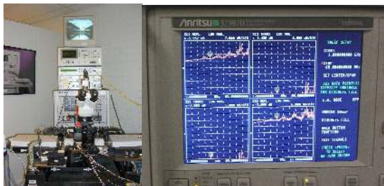
Figure: VNA (Vector Network Analyzer) and VNA screen showing the magnitude of the S -parameters for a 2 port.
