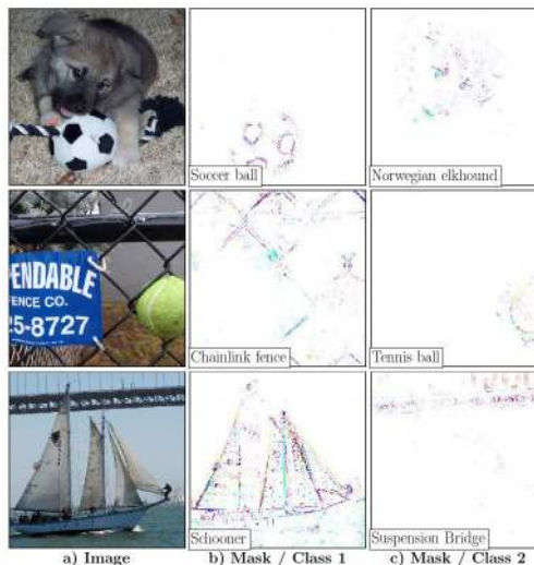
Figure 4: Explanation masks for images with multiple objects computed using the deletion game and GoogleNet . FGVis produces class discriminating explanations, even when objects partially overlap. Additionally, FGVis is able to visualize fine-grained details down to the pixel level.
