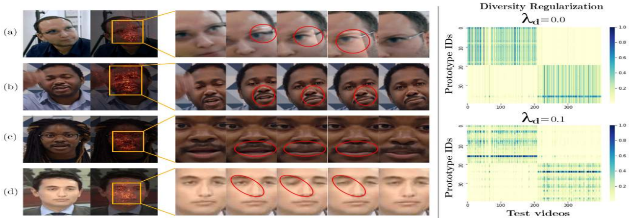
Figure 4. Visualization of learned dynamic prototypes. Left column depicts the different classes of temporal artifacts and unnatural movements found by DPNet. Right column shows the effect of diversity regularization (7) on prototype similarities across test videos.
