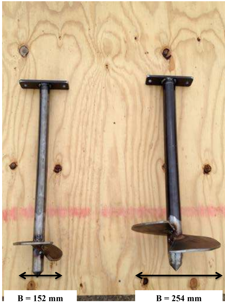
Figure 5: Test anchors (B = 152 mm, Total Length = 597 mm; B = 254 mm, Total Length = 616 mm).
