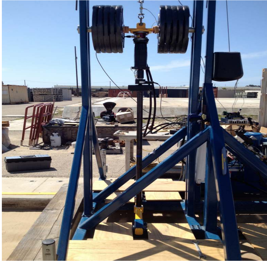
Figure 10: Helical anchor load frame.
