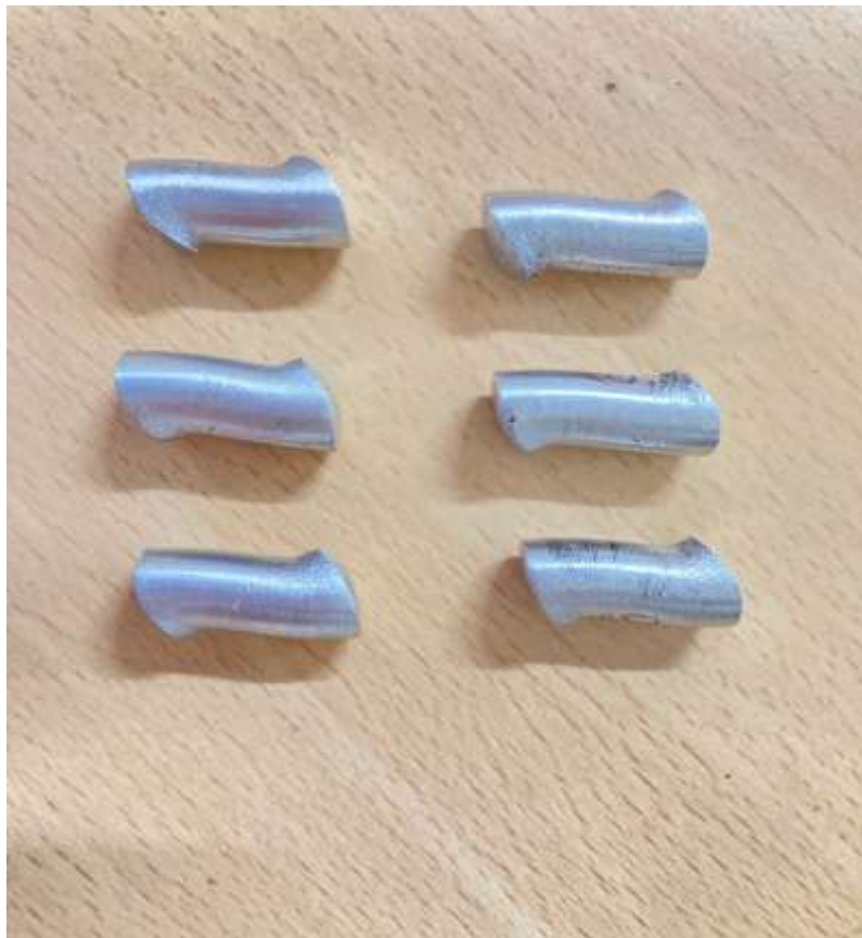
Fig. 1. Compressive strength composites samples of Al-Mg-Cr alloy reinforced nano WC ceramic particulates
