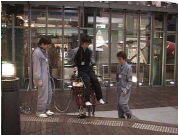
Fig. 15 WL-16R II carried a person to climb steps in Hakata Riverain shopping mall
