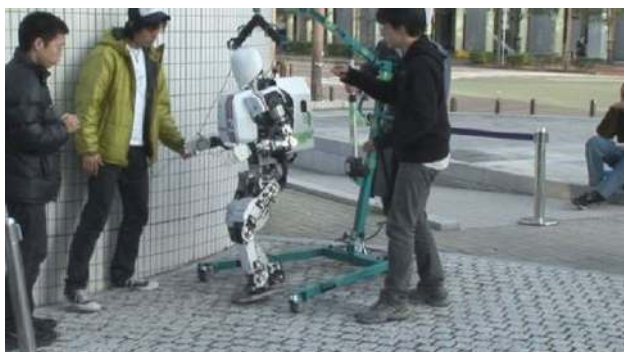
Fig. 11 WABIAN-2R walked on the bumpy surface with tiles angled 2^{\circ} – 5^{\circ} (forward-axis) down (experimental site no. 7)
