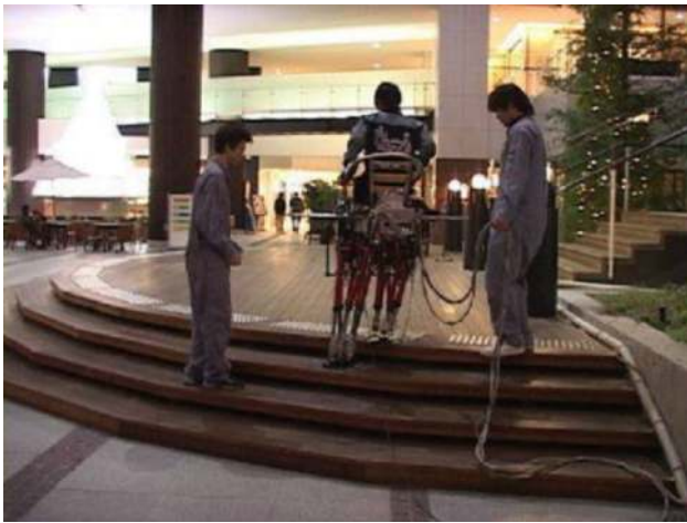
Fig. 14 WL-16R II carried a person to climb steps in Hakata Riverain shopping mall
