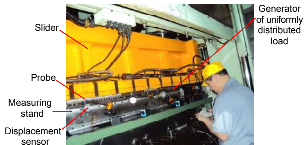
Fig. 9 Measurement of prototype's linear deflection
