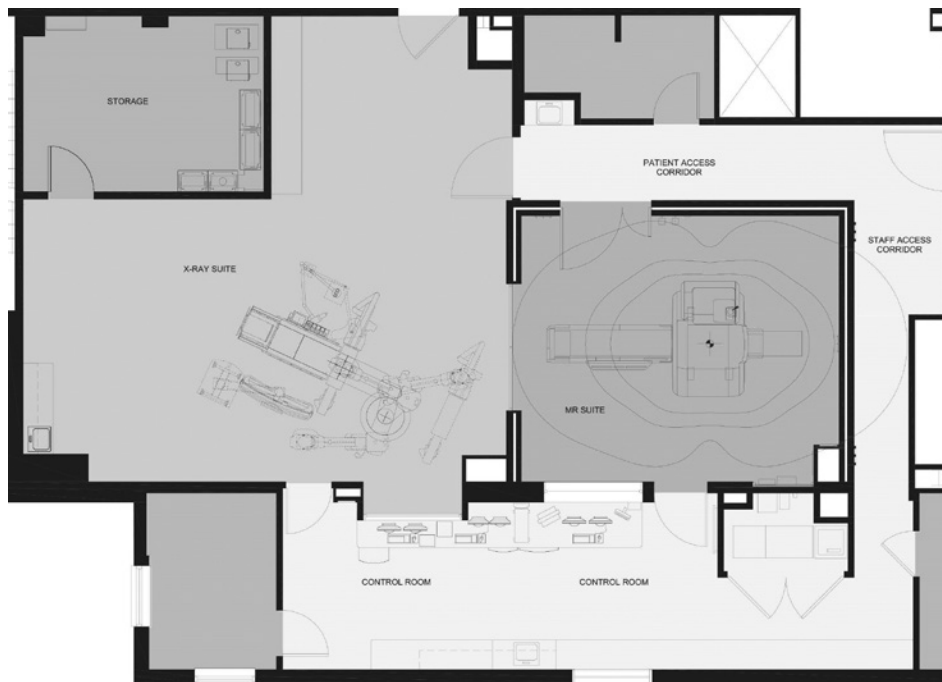
Figure 1. Floor plan of the National Institutes of Health hybrid magnetic resonance (MR) cardiac catheterization lab. Image courtesy of Christopher Dail, project architect, National Heart, Lung, and Blood Institute, Bethesda, MD.
