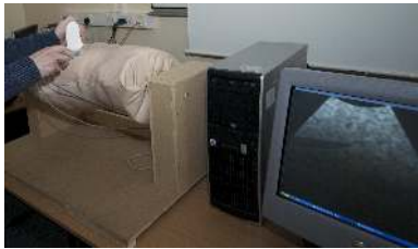
Fig. 6 Mannequin ribcage synchronised with the virtual environment (3D meshes and ultrasound rendering)
