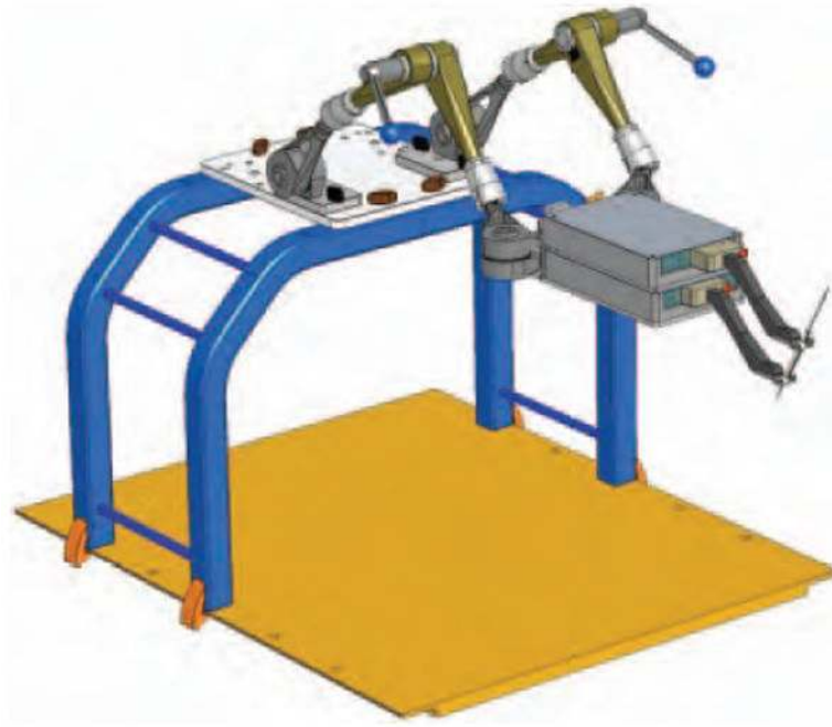
Figure 6. Biopsy robot II in a 2 by 2 degree of freedom configuration mounted on two passive holding arms.
