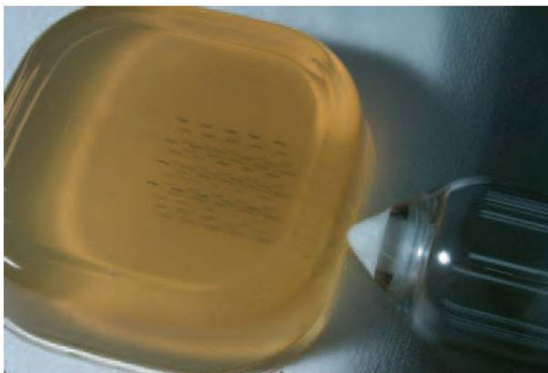
Figure 15. A 4x4 pattern of seeds with 10 mm spacing automatically placed in agar shows average seed placement errors of 0.652 mm.
