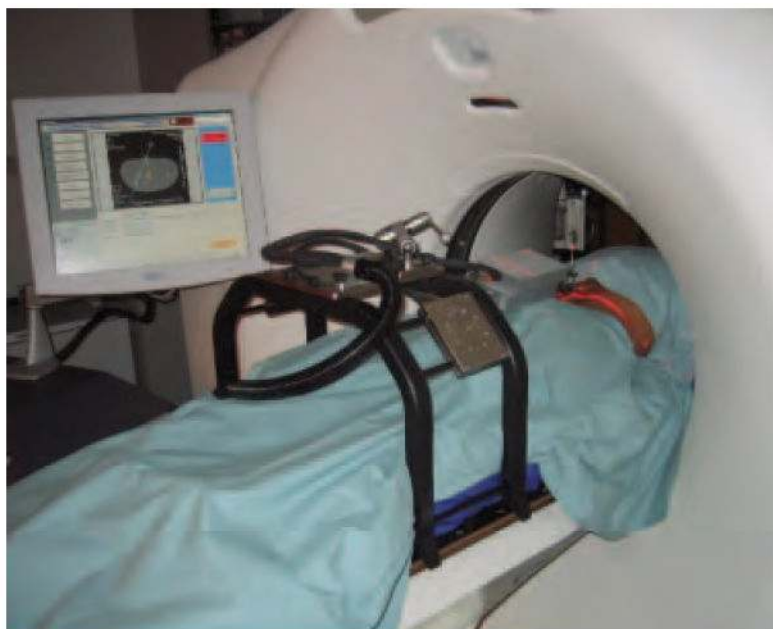
Figure 7. Biopsy robot II during initial phantom study.
