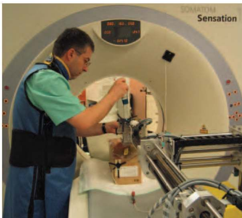
Figure 4. Biopsy robot I during in vitro testing for image-guided interventions under CT fluoroscopy.
