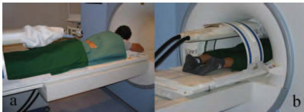
Figure 8. (a) INNMOTION robot for MRI-guided procedures; (b) moved into the bore.
