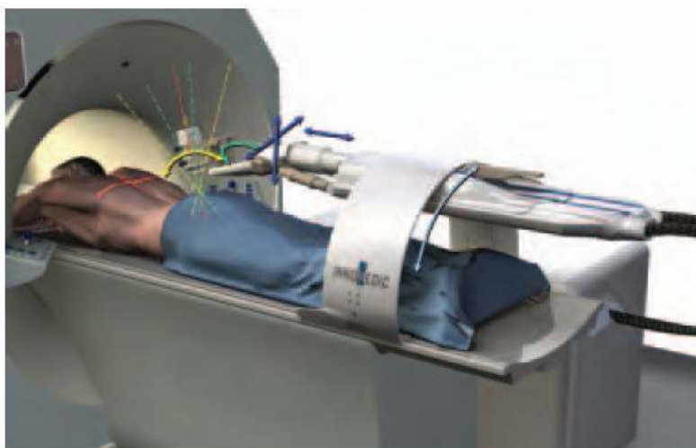
Figure 10. INNOVATION with six degrees of freedom can be mounted on different types of MRI patient beds.
