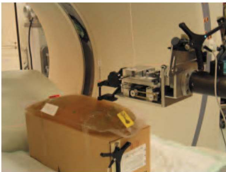
Figure 5. Close-up of testing showing phantom (peas can be seen in the bag), needle positioning unit (NPU), and optical trackers.
