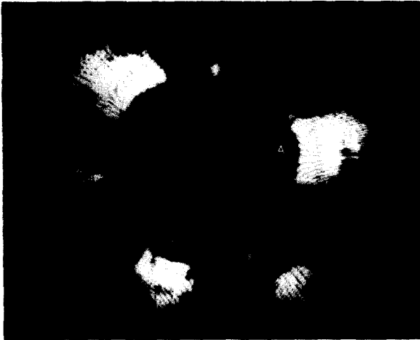
Fig. 10. First image obtained in vitro using the catheter shown in Fig. 8. On this image only the very strong echoes from the cage construction (A) and a plaque (B) are displayed.
