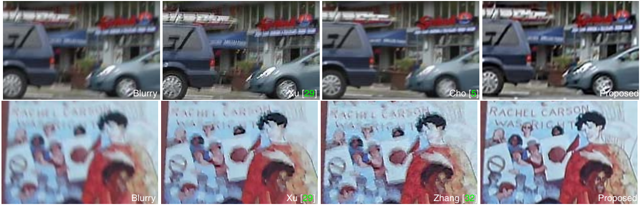
Figure 8. Video deblurring results on the car (top) and mural (bottom) sequences. The deblurred frame from the proposed method has more fine details and fewer ringing artifacts compared to the results from single frame image based deblurring method such as [29] and [32], and is sharper than the result from [5].
