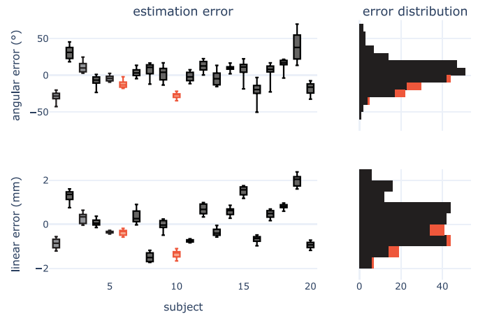
Fig. 9. Error of the linear (bottom) and angular (top) insertion depth estimation per subjects (left) and the corresponding histogram (right). Partially inserted subjects are highlighted in red.
