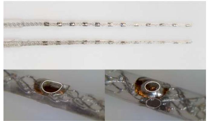
Fig. 2. The Flex 28 electrode array in two orientations (top) and photomicrographs of a single (bottom left) and double (bottom right) contact pads with highlighted outline.
