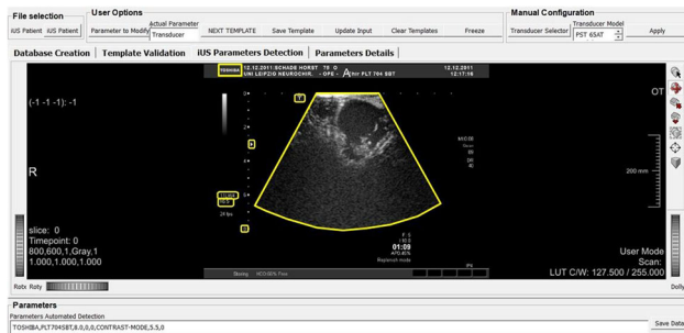
Fig. 2 The identified parameters are shown into the text box on the bottom left corner. They are: the US device model (Toshiba), the transducer (PLT704SBT), the image depth (8.0 cm), shape (0 for trapezoid) and orientation (0 when the marker is on the left), the imaging mode (CONTRAST) and the frequency (5.5 MHz)
