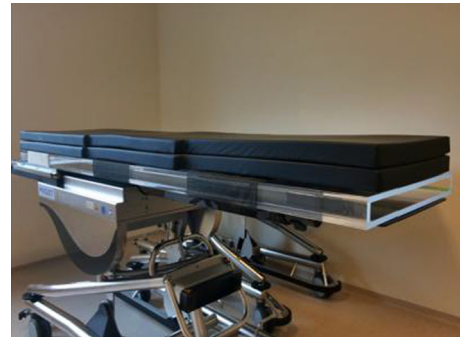
Fig. 2 Adjusted operating table (OR) that combines X-ray “transparency” of carbon OR tables and electromagnetic (EM) tracking with NDI Tabletop Feld generator (left image). This is a combination of the Magnus carbon system (MAQUET, Germany) and a custom-made Perspex sleeve for positioning of the EM field generator
