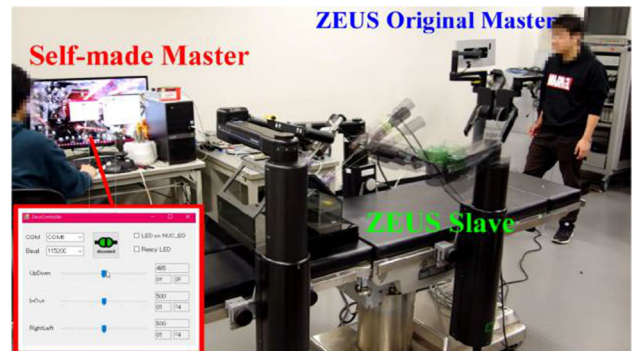
Fig. 2 This figure shows the result of manipulating the ZEUS slave via ORiN from a GUI application developed as a self-made master
