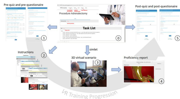
Fig. 1 The task list assembled by the author auto-initializes the VR training progression including: pre-quiz and questionnaires, instruction pages, the interactive haptic virtual simulation scenario, the proficiency report, and the post-quiz and questionnaire
