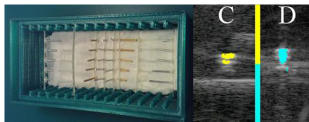
Fig. 1 Experiments with the specially developed and 3D-printed phantom. Left: photo of the phantom (with dimensions mm 3 ). Right: component C most apparent on a plastic rod in ethanol and component D observed upon aluminum rod in water
