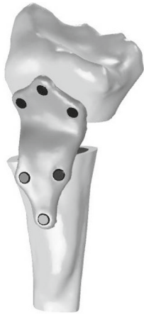
Fig. 2 The novel patient-specific plate design. Screws are arranged in a triangular pattern to counteract torsional moment
