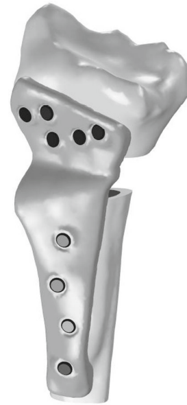
Fig. 1 Patient-specific plate initial design. Screw configuration and plate thickness are similar to standard anatomical plates
