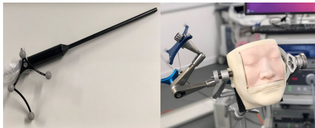
Fig. 1 A novel pituitary probe for transsphenoidal surgeries for intraoperative ultrasound imaging and Kezlex anatomical model (Ono & Co., Tokyo, Japan) in a Mayfield clamp (Integra, Saint Priest, France)
