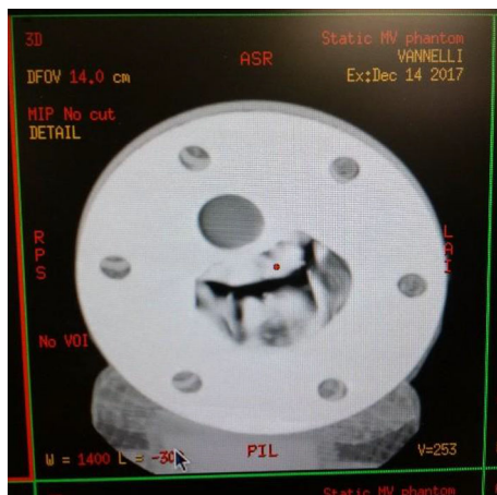
Fig. 1 3D volume rendering of silicone mitral valve arrested at the first time point (pre- to mid- P wave)
